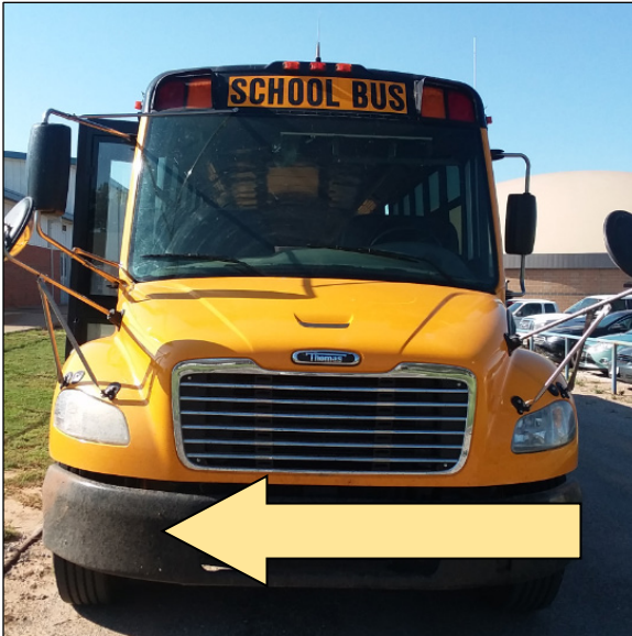
Missing Crossing Arm
